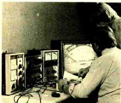
A HIGHLIGHT OF THE RECENT SENCORE troubleshooting seminar was the company's all-in-one AM/FM/stereo and CB analyzer, developed to help service in-dash combo units.
