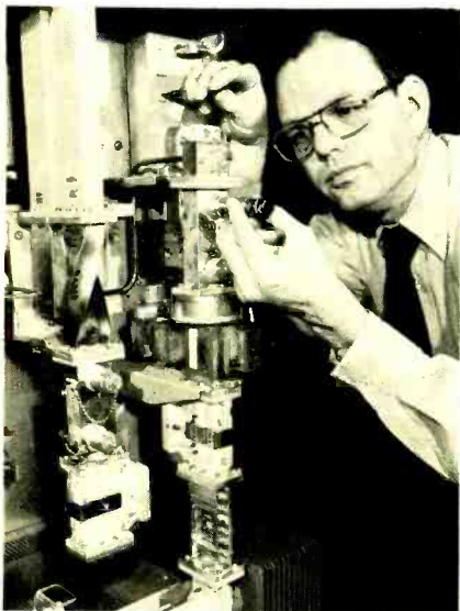
PART OF THE AR6A SINGLE SIDEBAND microwave transmitter, with one of its designers, Bell Laboratories engineer William Robinson.
